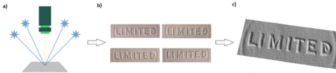
Fig. 1. (a) Illumination geometry for PS, (b) 4 images obtained with different angles of illumination, (c) results of PS algorithm to generate 3D surface map.
